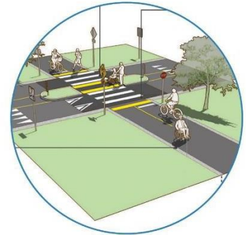
Illustration of a shared use path, a separate path from motorized traffic.
